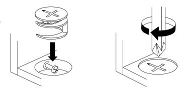
Turn cam lock clockwise to tighten.
